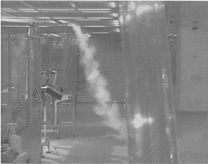
FIGURE 7 Visualizing airflow under a laminar flow unit.
