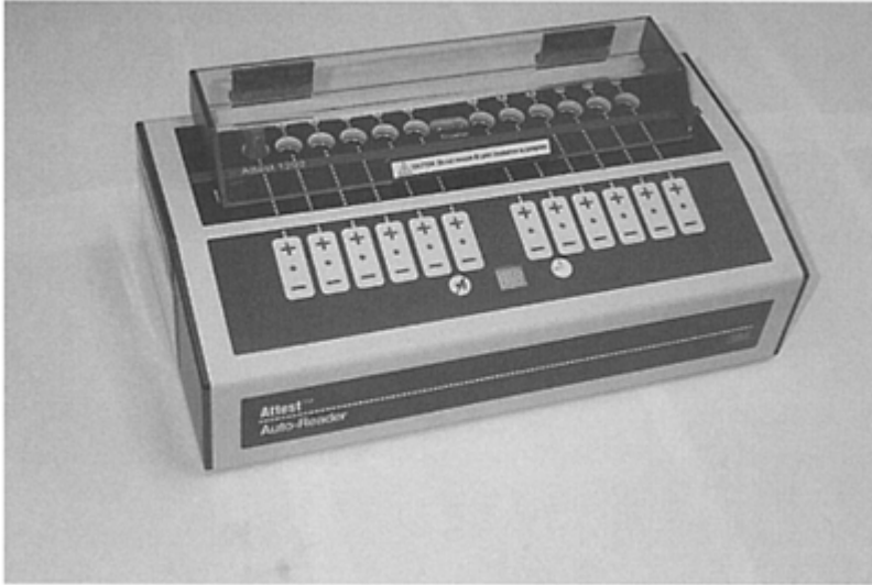
FIGURE 4 An example of a fluorometric reader for detecting the presence of active alpha-glucosidase enzyme.
